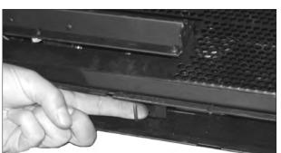
Figure 7: Adjusting the venturi air setting.
